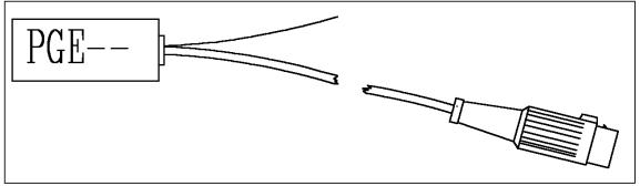
This interface is used in cars with electronic speedometer. It is connected to the original pulse generator of your car in accordance with a separate instruction.
